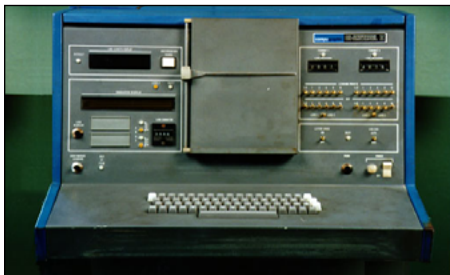
This is the Compugraphic Machine that produced lines of text to be pasted up.
